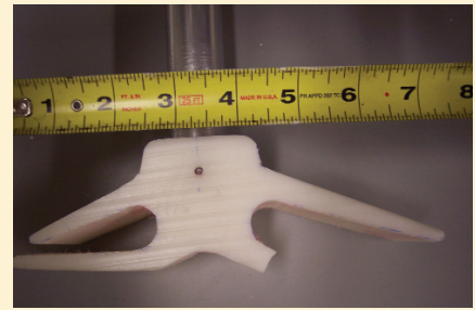
Fig. 3 — Plastic foot-to-aluminum stem joint prototype which failed during fatigue testing after two-million cycles.
