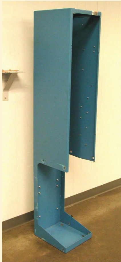
Fig. 2 — Adhesively bonded cabinet during seismic testing at Southwest Research Institute.
