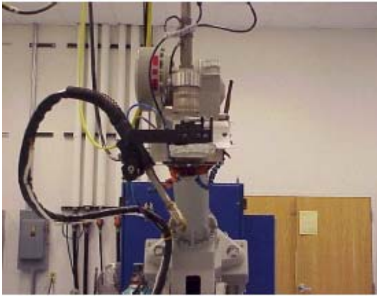
Figure 3. View of the motion system (attached to a welding robot) – can be mounted on a simple side-beam carriage as well
